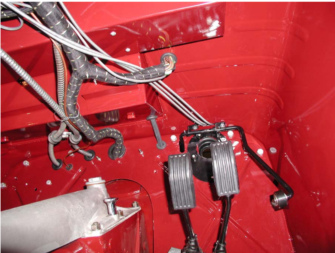
There is lots to see here. Carpet pegs, tach & speedo routing, clips & grommets, battery cable, control cables to engine compartment, and accelerator linkage.
