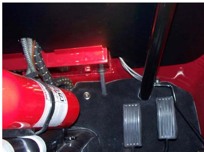
Grouping the cables, harness, and oil pressure line and then the engine cables will give you a nice organized install.
