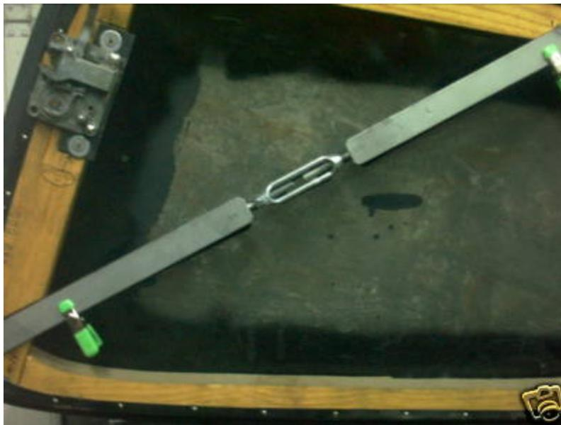
Each turnbuckle body is marked with the letter “L” on one end. Similarly two of the straps are marked with the letter “L” on the back. These components have “left hand” threads. The first step is to screw each strap marked with “L” into each turnbuckle end marked with the “L”. Next screw the nuts onto the remaining straps then screw the remaining strap into the other end of each turnbuckle.
