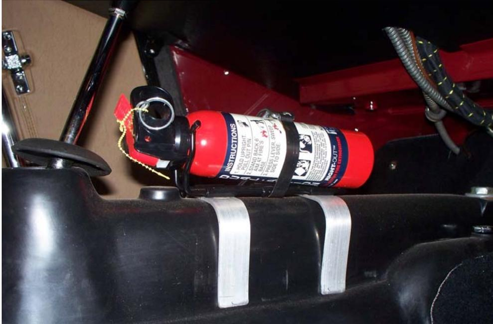
**Fire Extinguisher Brackets:** These brackets easily on most portable fire extinguishers. They are designed to be used in the TC without drilling holes in the car. The “u-shaped” mounts place the extinguisher out of the way, but accessible, on top of the rubber gear box extension tunnel cover forward of the gearbox shift lever. The width is designed to gently grip the sides of the cover without damage to the cover.
