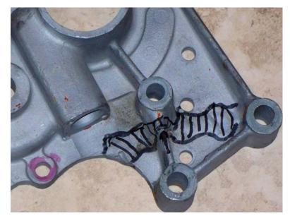
This photo shows the high fail area. The black hashed area overlays what has been previously repaired (welded)
