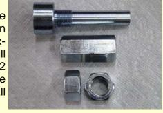
2. Place the flat copper washer in the top of the extension. Then screw the MC body onto the extension using your hands to tighten. Just a strong grip and turn of the hands should be adequate.
