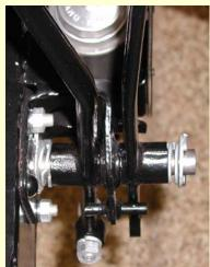
There may be occasions where you still may not be able to get the pushrod out. If so, you will have to remove the pedal shaft to remove the brake pedal. Remember to do so; you have a cotter pin on each end of the shaft next the flat washer. Then the pedal shaft can be driven out through the hole in the chassis frame.
