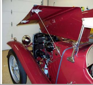
Once the bracket is installed simply raise the bonnet and place the "nut" end of the rod in the bracket and the rubber ball inside the round spring associated with the bonnet latch.
