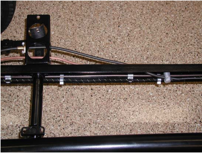
5 – Install fuel lines first. Harness sits on top.
