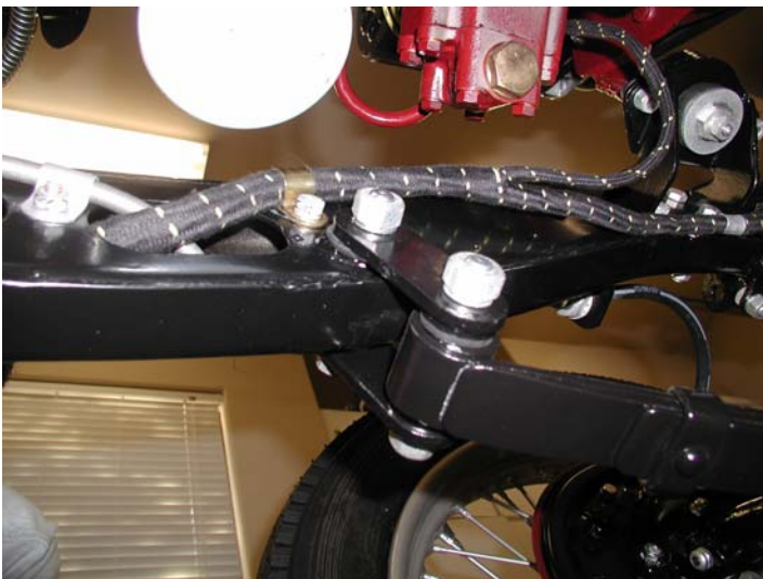
9 & 10 - Front left chassis routing with clip locations
