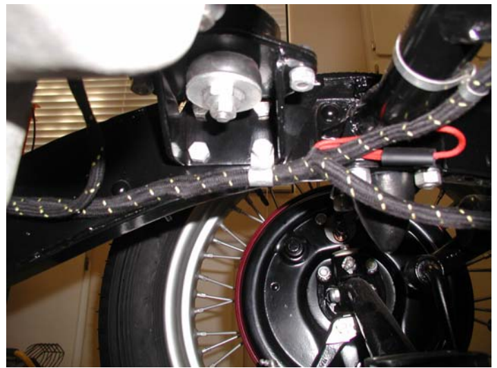
9 & 10 - Front left chassis routing with clip locations
