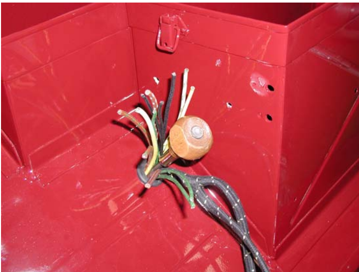
15 – Use an awl to make an opening to organize your wires by color
